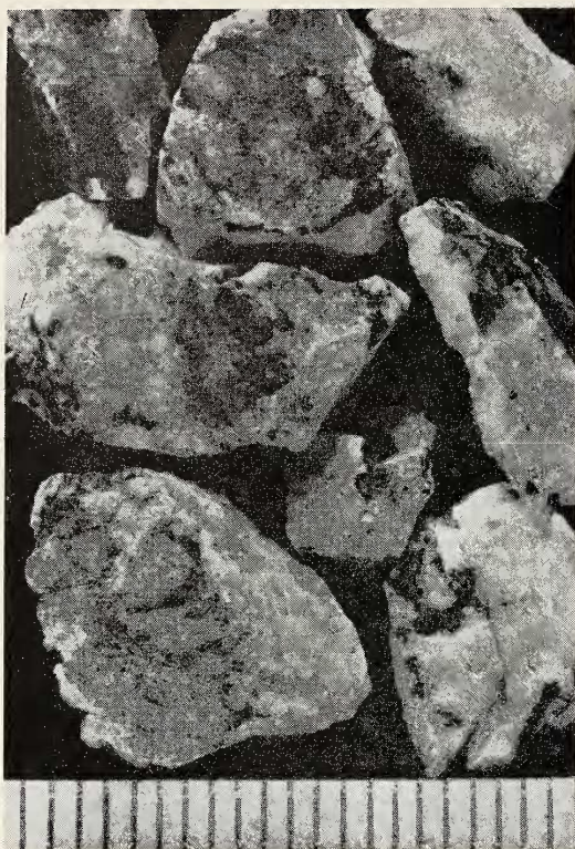
FIG. 1. Fragments of halloysitic veins from Haiku, Maui. Dark coatings are surface manganiferous deposits. Scale units in mm.
